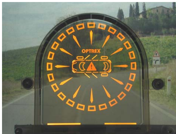
Transparent OLED signage device. Photo: Optrex Europe GmbH, Babenhausen, Germany
